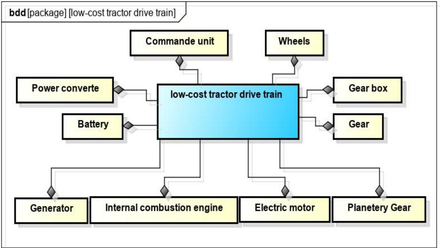
Fig. 3 Block definition diagram of the drive train of the low-cost tractor.
