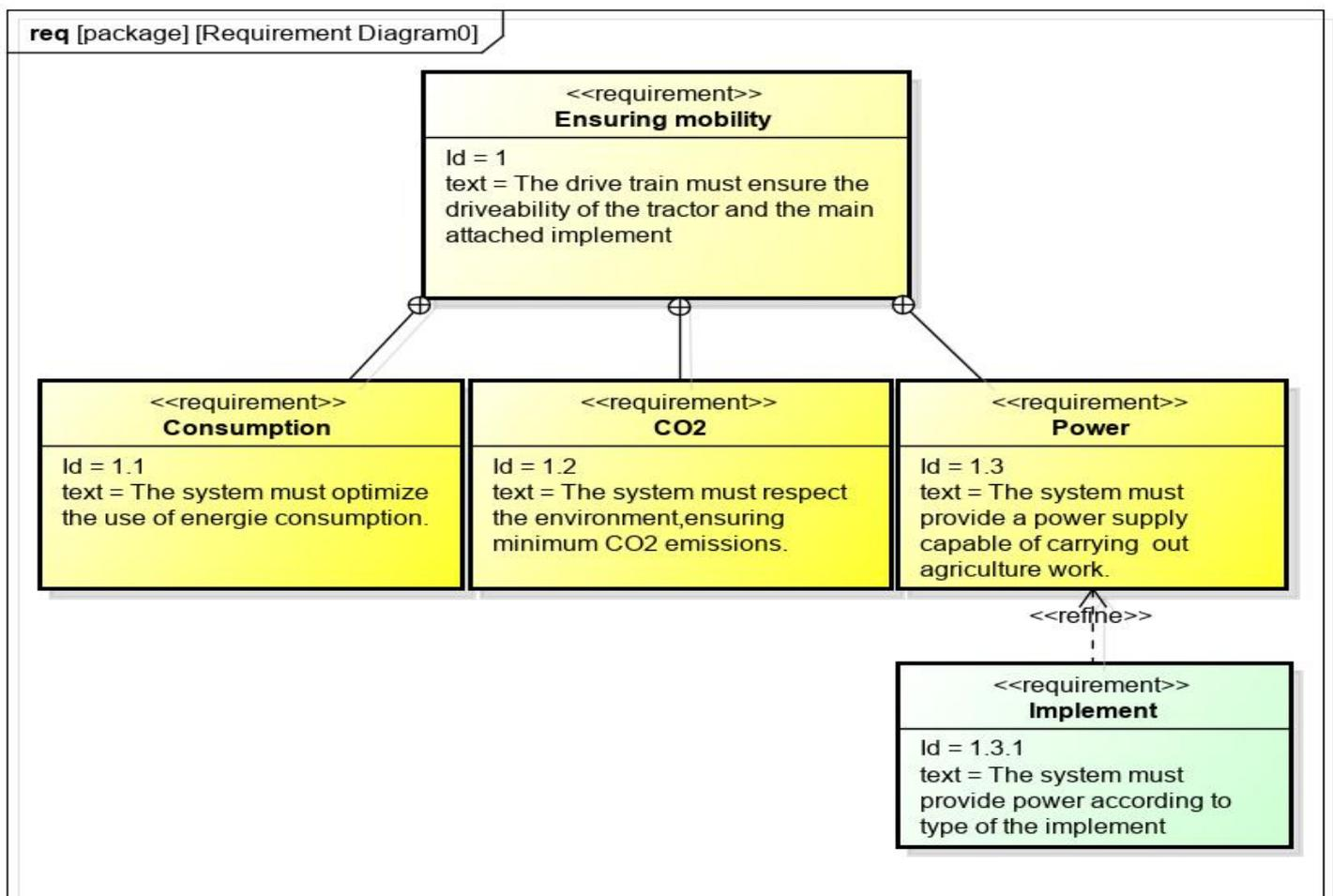
Fig. 2 Requirement diagram of the drive train of the low-cost tractor.
